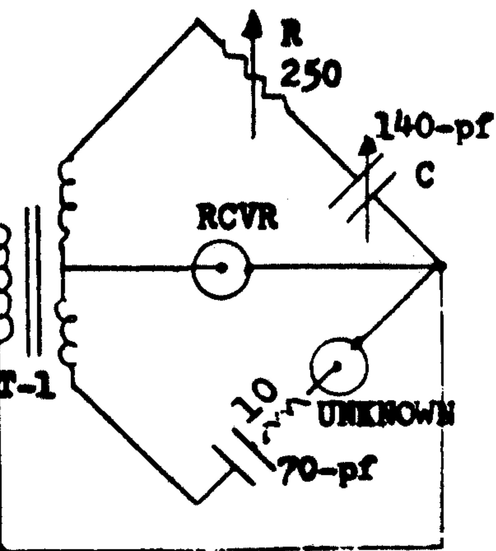
Reactance Chart. Refer to the schematic diagram on page 7. R and C are the panel controls labeled R and X. C = 70 pf at a dial reading of X = 0. There is a 70-pf capacitor in series with the unknown. If the unknown series resistance and reactance are  $R_U$  and  $X_U$  then at null.
